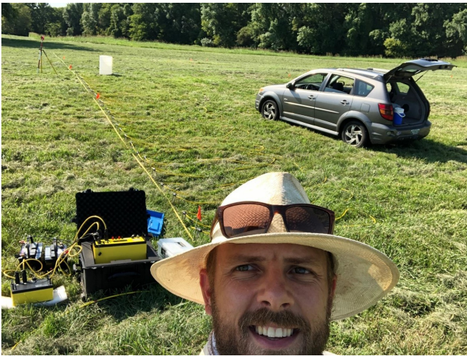
Grant Stauffer conducting electronic resistivity tomography.
